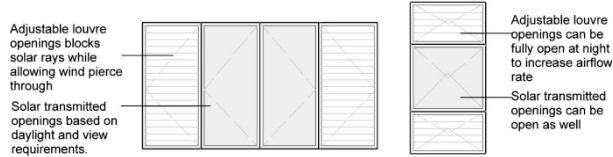
Figure10: Elevation detail for window examples with solar-excluded and solar-transmitted panes.
